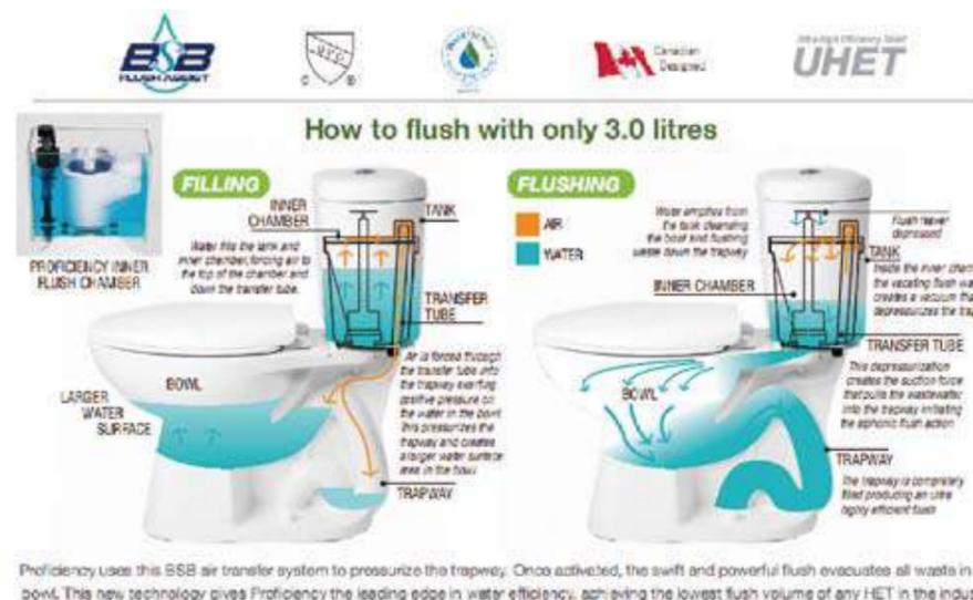
Proficiency uses this BSB air transfer system to pressurize the trapway. Once activated, the swift and powerful flush evacuates all waste in the bowl. This new technology gives Proficiency the leading edge in water efficiency, achieving the lowest flush volume of any HET in the industry.
